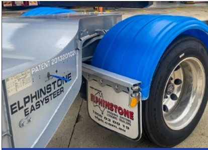
The leading axle in the EasySteer suspension steers at all speeds.
