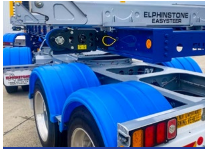
EasySteer trailers have Elphinstone Auto Air Tensioner winches with quick-release load restraint latches.
