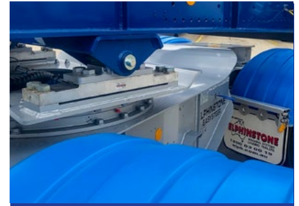
EasySteer trailers come equipped with loadcells to provide high accuracy weighing.
